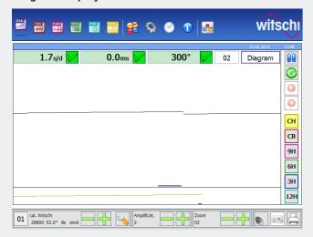
The rate deviation is continuously drawn on the screen. Measured values for rate deviation, amplitude and beat error are displayed numerically.
