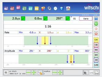
The Vario mode measures the rate and amplitude stability over a longer time range. Each numerical measurement is represented by an arrow on the linear scale. The following values are constantly updated as long as the measurement process is running:
