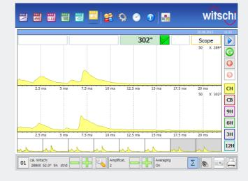
The Scope function graphically displays the acoustic beat noise of the watch. A detailed analysis of the beat noise, i.e. of the state of the escapement, can be carried out. The display can be switched from one to two horizontal axes. Thereby, the averaging of the signals of 1, 10, 20 and 50 beat noises is possible.
