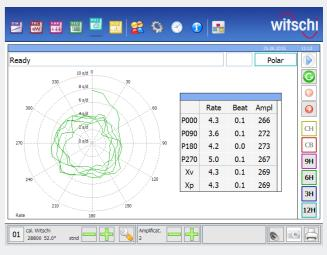
POLAR display mode indicates the rate stability in a polar diagram. One revolution (rotation time) of the Tourbillon watch corresponds to one revolution on the diagram. The average values of rate, beat error and amplitude for specific angles are calculated and displayed. The watchmaker can now determine the centre of gravity of the balance wheel. This world first makes the Chronoscope X1 the most comprehensive watch measuring and testing device of all time.
